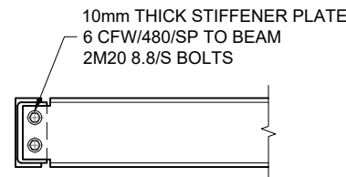
STEEL BEAM CONNECTION - 200 PFC TO 200 PFC 180 PFC TO 180 PFC SIM. (CONNECTION CAPACITY 55 kN ULTIMATE) ALTERNATIVELY SITE WELD USING 6 CFW/480/SP ALL ROUND
